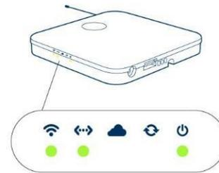
When the Gateway is ready, a minimum of 3 green lights will light up on the side of the Gateway. There will also be a white light lit up on the front of the Gateway. This indicates that the Gateway is ready to be connected to your app.
